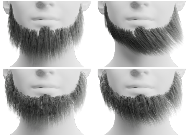
Figure 9. Time evolution (from left to right) of facial hair simulated using MS (top) and AMS (bottom). Our augmented formulation introduces key interactions that preserve the intended structure of facial hair throughout the simulation, while in MS, strands lose their overall form at initialization.
