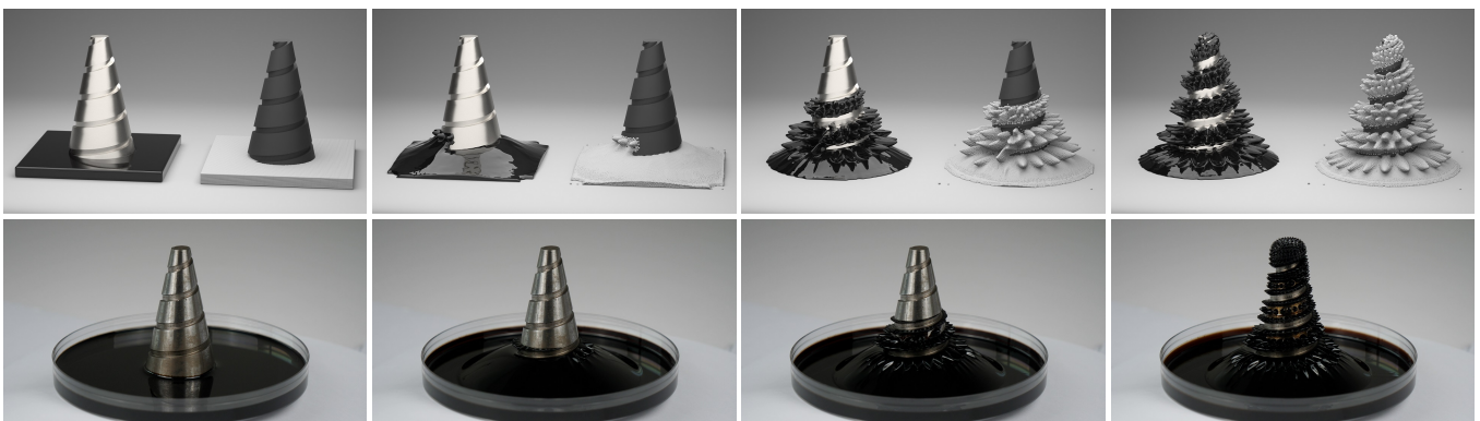
Fig. 17. We make use of the same steel helix as shown in Figure 16 which is magnetized in order to attract ferrofluid from its base to its top. The ferrofluid is literally climbing up the helix as the field strength increases as shown in this real experiment (bottom row). The simulation (top row; left: final rendering, right: particle view) can reproduce this observation as presented here.
