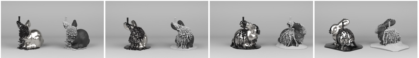
Fig. 15. We are able to simulate magnets of arbitrary shapes. In this example, the geometry of the well-known Stanford bunny is used. The magnetic bunny is showered with ferrofluid which is forming its characteristic spikes and patterns on the surface. The final rendering is shown on the left side of each frame while a particle view is presented on the right side.
