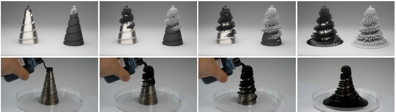
Fig. 16. In order to allow for a qualitative comparison with complex geometry, we perform a real experiment (bottom row) in which we pour a ferrofluid down the top of a steel helix placed above a strong electromagnet. Our simulation (top row; left: final rendering, right: particle view) leads to a visually comparable result.
