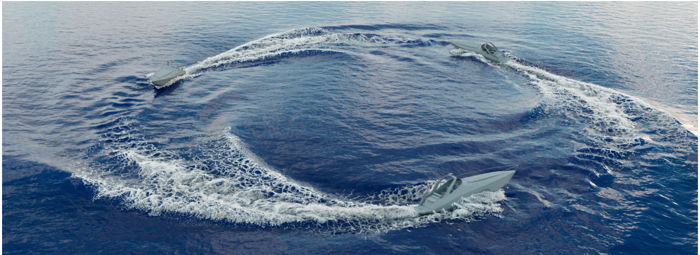
Fig. 1. Photorealistic rendering of a simulation comprising three speedboats riding in a circle on the ocean computed with our hybrid approach combining FLIP and BEM.
