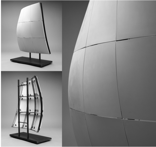
Fig. 14. Photos of the facade composed of 3 \times 3 panels fabricated with our flexible mold. Please zoom in for a closer look at the surface.
