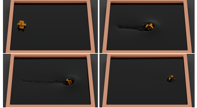
Fig. 16. Meteor (Viscous). A meteor hitting into a tank of viscous liquid. The grooved trajectory by the meteor is gradually smoothed. The dynamic viscosity coefficient is \mu = 5\,000\text{ Pa}\cdot\text{s} . The domain size is about 30\text{ m} \times 30\text{ m} \times 2\text{ m} and the grid resolution is 0.05 m.
